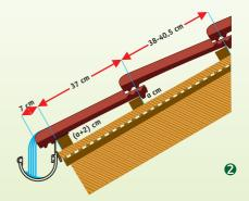
Recommended minimum roof slope using covering (eg membrane): 30% (17°)
