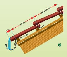
Recommended minimum roof slope using covering (eg membrane): 30% (17°)
