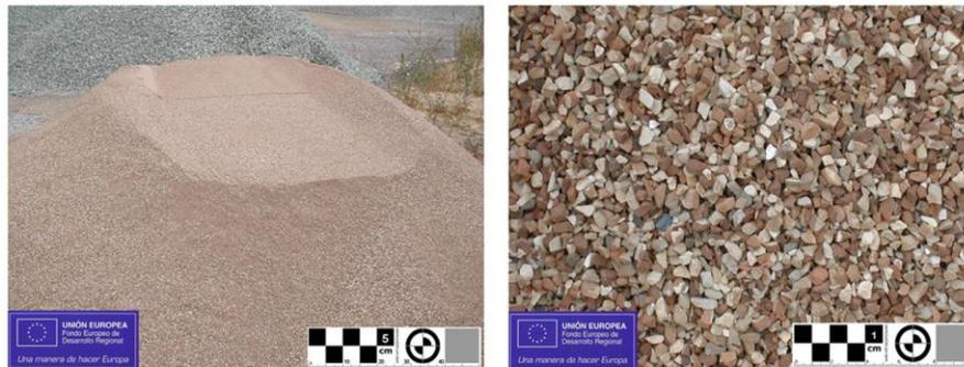
Figure 2 – Recycled ceramic aggregates. Source: Silvestre, R. et al., 2013
